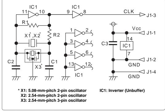
Figure 3.5 Circuit of the oscillator board (OSC-2)
